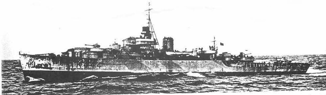
Matane, January, 1944, typical of the first 15 RCN frigates, with single 4-inch forward and no clinker screen to her stack
